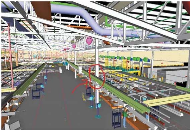
During a 3-D model review of the plant, interference between the already-installed columns and a process conveyor was flagged.
