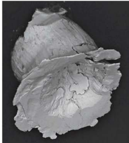
This low-alloy-steel particle of 120 \mu\text{m} (4700 \mu\text{in} ) diameter was found in a diesel-injection nozzle. Forensic examination of various components in the system after rinsing led to the conclusion that the debris originated in the high-pressure pump.
