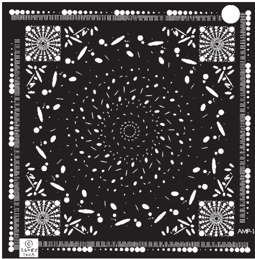
Figure 5 – The PGS specimen is fabricated with five distinct analysis zones. The four corner zones each contain 1092 circular features ranging from 1 to 100 microns in diameter and are intended for quick system checks. When combined with the central array of elliptical features, a 4x4 mm zone of 5050 features is available for more comprehensive tests.
