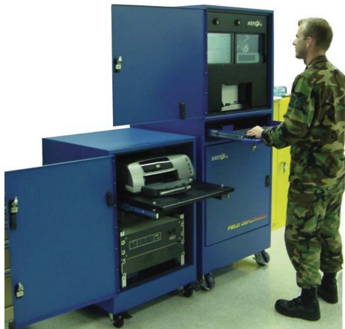
Figure 1. The JEMM is a self-contained and ruggedly packaged automated SEM/EDX unit that is deployed by the US Air Force in support of aircraft squadrons.
